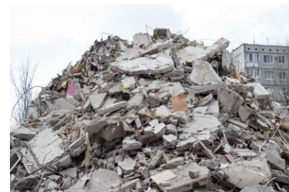
Construction debris as aggregate
