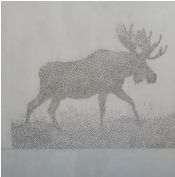
The graphical surface when using colored concrete
