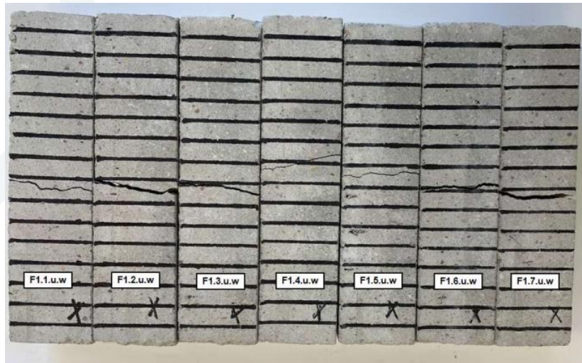
Fracture pattern after 3-point bending – test orientation 'u-w'
